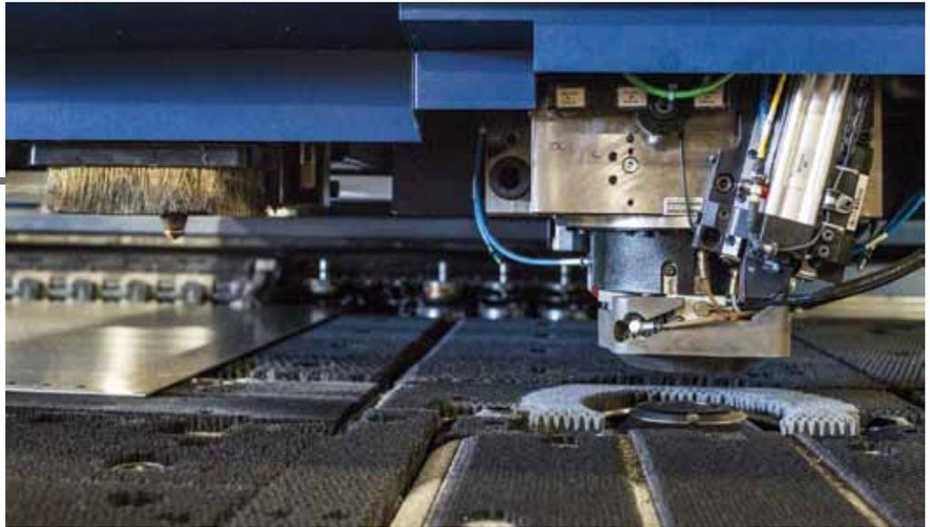
on the floor because we can do all the tapping on the machine. They work in a different area now. They used to do just tapping. It is more precise as well, we break a lot less taps than with the manual method. It expanded our production and the quality is much higher.” Another benefit to this machine is the Sheet Master automatic loader. “We can load up the sheets and it will run by itself. It is fully independent,” said Charest.
