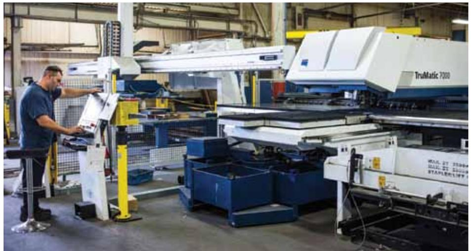
The TRUMPF TruMatic 7000 punch laser combination machine is a recent addition to the company's cutting and bending operations. Sébastien Charest says it gives Groupe Ultra a competitive edge.
