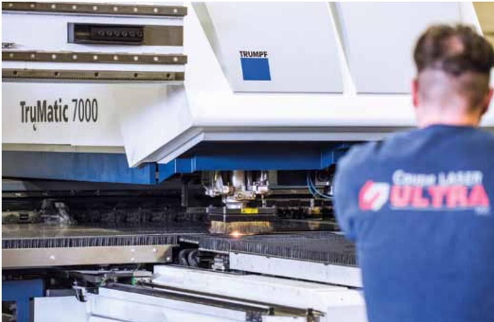
Able to hold 22 tools, the punch laser combo machine's punching head has a maximum stroke rate of 1,200 1/min in the medium format (1,000 1/min in large format).
